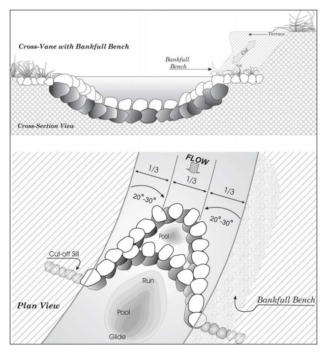
Figure 8. Example of a boulder Cross-Vane and constructed bankfull bench.
