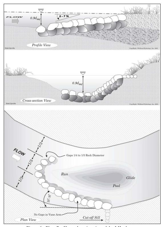
Figure 6. Plan, Profile, and section view of the J-Hook vane.
