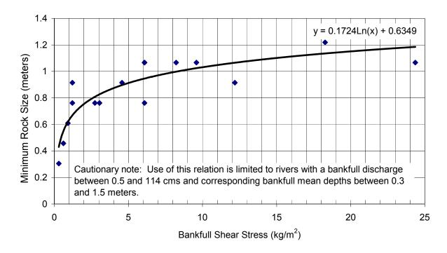
Figure 10. Minimum rock size as a function of bankfull shear stress.
