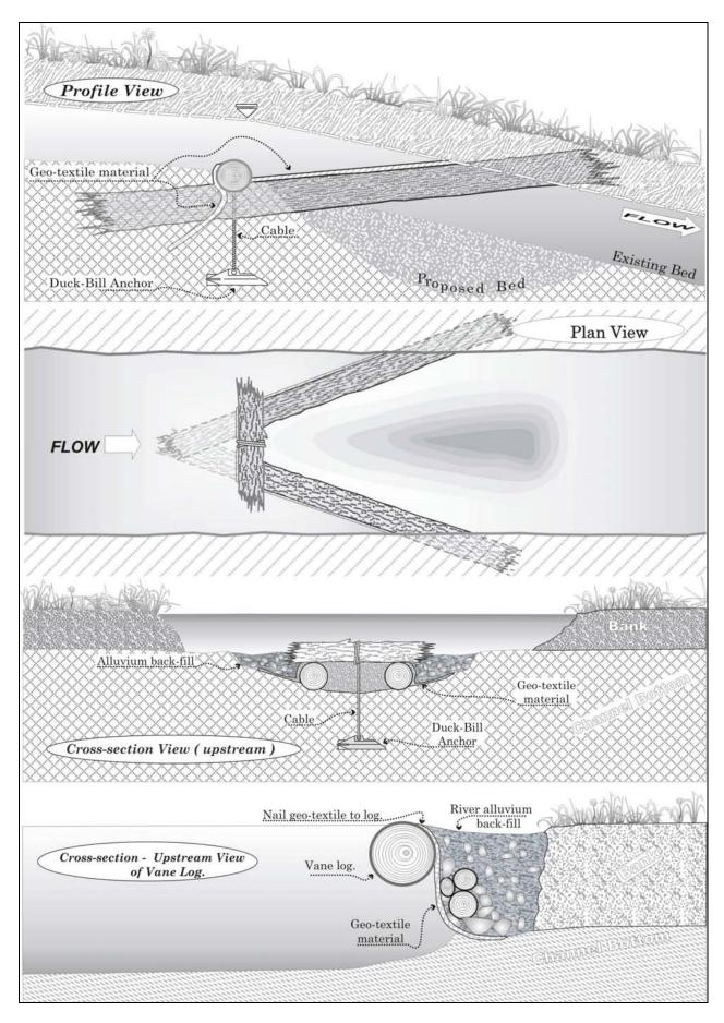
Figure 11. Cross-Vane using logs and a duck-bill anchor.
