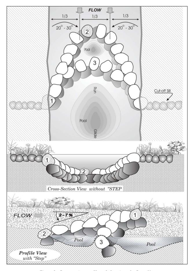
Figure 3. Cross section, profile and plan view of a Cross-Vane.
