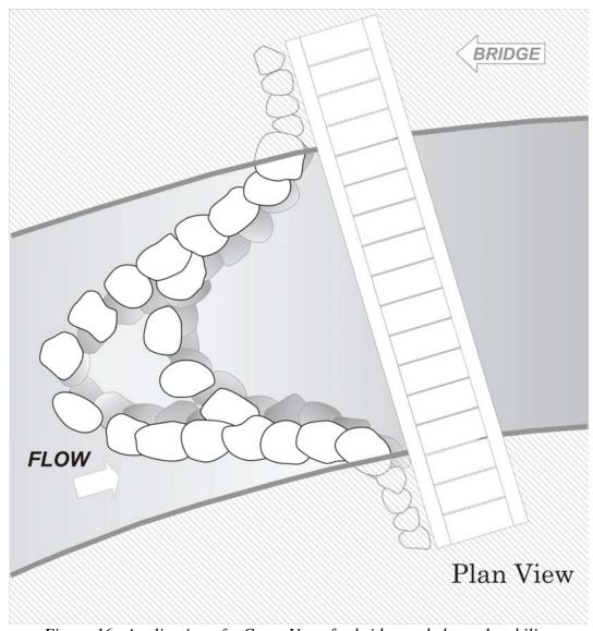
Figure 16. Application of a Cross-Vane for bridge and channel stability.
