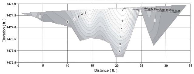
Figure 12. Velocity isovels of a J-Hook Vane, at Turkey Creek, Colorado. (Velocity in Ft./Sec.)
