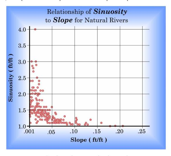
*Figure 1. Relation of sinuosity to slope for natural rivers.*
