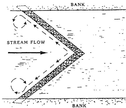
Fig. 12. V shaped gravel trap (Reeves and Roelofs, 1982).
