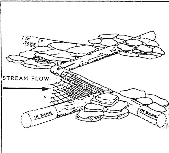
Fig. 2. Low stage check dam (Seehorn, 1985).
